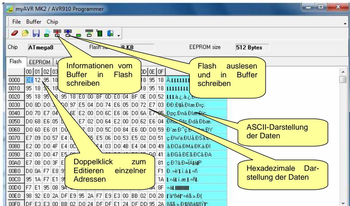
The screenshot shows the 'myAVR MK2 / AVR910 Programmer' window. The 'Flash' tab is active, displaying a table of memory addresses and their contents. The table has columns for address (0000 to 00F0), hex values, and ASCII characters. Yellow callout boxes are overlaid on the interface:
