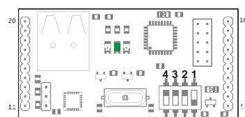
myMode for TWI- and SPI-communication (activate via software)
